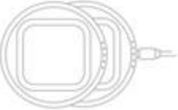
**2** Stack batteries on charging base, lining up Pogo pins to trigger flashing LED
